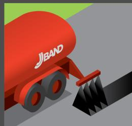
Apply J-Band at the time of construction to reduce permeability under the surface where centerline rumble strips will be installed.
