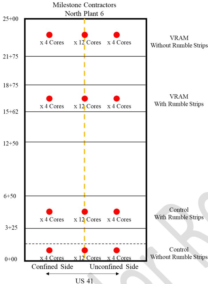
Figure 2: Lowell test section layout.
