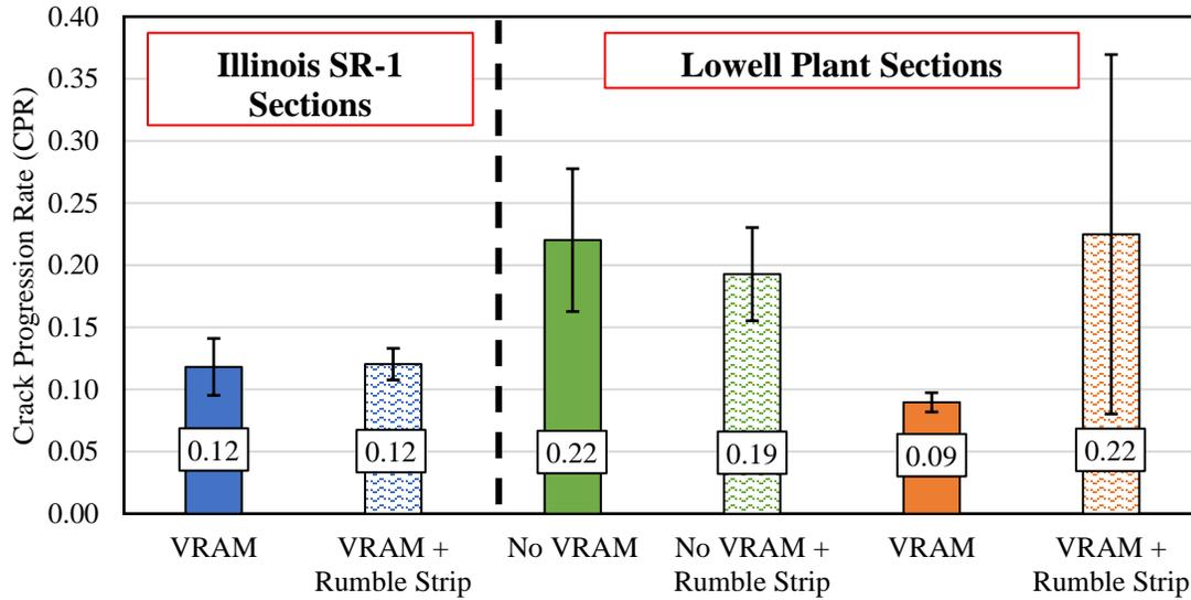
Figure 13: Summary of crack progression rate results from overlay testing for Illinois SR-1 and Lowell Plant test sections with error bars denoting one standard deviation.
