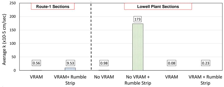
Observed minimal to no permeability of cores that contain VRAM.
