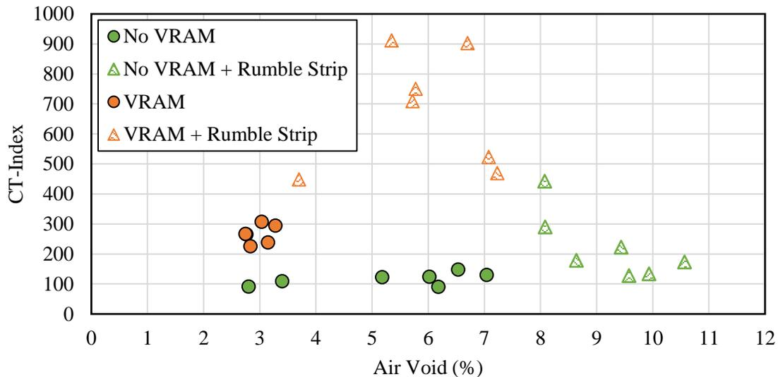
Figure 12: CT-Index results versus measured air void on cut specimens from Lowell Plant sections.
