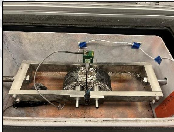
22 Figure 7: DCT test set up.
