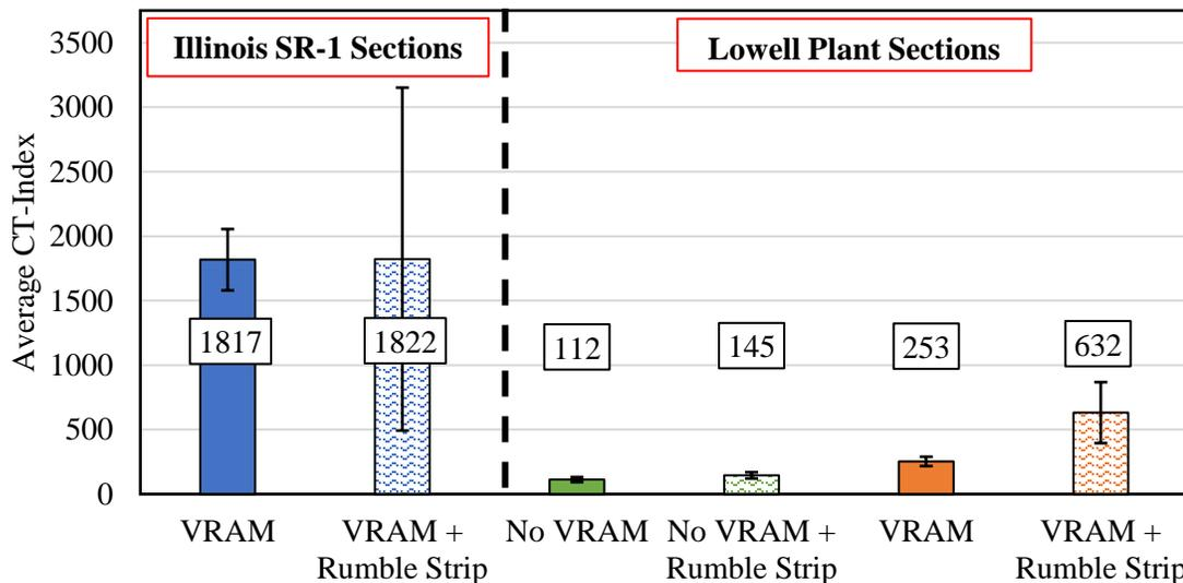
22 Figure 11: CT-Index results on field cores from centerline joint cores only along Illinois SR-1 and Lowell
