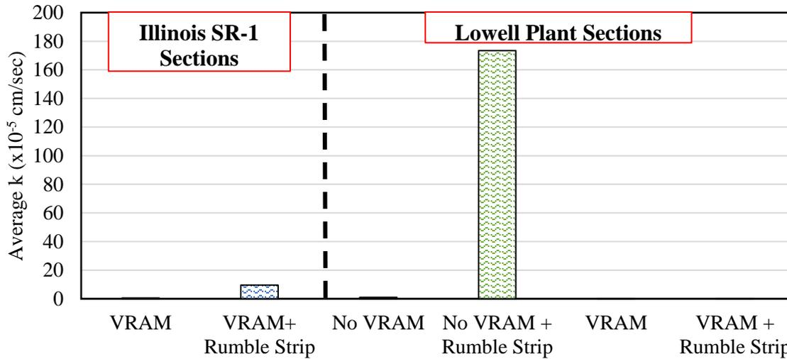
Figure 14: Summary of lab permeability results for Illinois SR-1 and Lowell Plant test sections.
