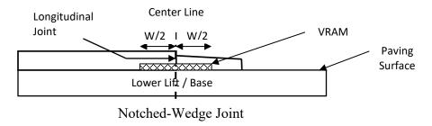
The VRAM shall be applied in a single pass placed by any application method listed in the Equipment section. VRAM application temperature shall not exceed 330°F.
